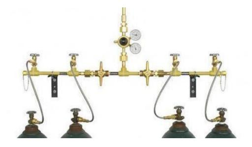
WST offers gas manifold system for oxygen gas supply to the panel. To achieve uninterrupted gas supply to the control panel, series of six cylinders can be connected to the mainfold system with one outlet supply. The system has flexible hose supply with opening valve, NRV, double stange regulator and pressure gauges. The thread size offered is as per Indian gas cylinders however connectors can be offered to meet load thread requirements, if customer give thread details.
