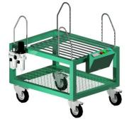
A portable trolley is offered for mounting control panle, placing powder feeder, vaporizer, gun mount stand, air control unit and storing hose sets. The trolley is constructed from heavy duty pipe and sheet metal construction for strength & rigidity. Four heavy duty castors are offered for the ease of movement of the trolley at site on the floor. Trolley is designed to meet asthetic looks and engineering strength.
