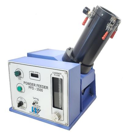
A volumetric metering type powder feeder unit if offered to feed the gun with coating powder from feeder canister outlet. The powder canister is designed to have top lid with viewing glass to see the level of powder and to charge the powder in the canister. The feeder is designed to have tilting canister assembly for easy emptying of the powder from the canister without removing the canister from the body. The feeder has rotameter type flowmeter for measuring carrier gas flow readout.
