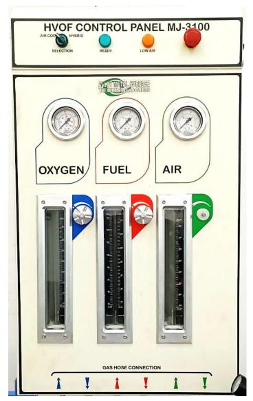
The MJ-3100 control panel is designed & offered controls, semi-automatic monitoring а and operation of WST gas-fueled HVOF thermal spray systems MACHJET-I. Offered control panel is user friendly and is provided with gas flow meter / rotameter for Oxygen & Compressed air. Operator Fuel, can easily adjust the knob to regulate the flow and set the float to the desired value on the twin scale shows flow range in NLPM/SCFH.
