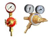
Gas control unit consists of two regulators viz, each for Oxygen & Fuel. Oxygen regulator is double stage type and can be easily mounted on the respective cylinders. The two stage regulator drops high gas pressure to the permissible pressures for the HVOF spray process. Each unit has two pressure gauges, for cylinder inlet pressure and regulator outlet pressure respectively.
