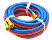
A twin hoses type set is offered for fuel and oxygen and pneumatic rubber hose for compessed air. The unit is offered in two length viz, 7.5 mtrs from flowmeter to the gun and 3 mtrs from cylinder to the inlet of flow meter. Both ends of the hoses are provided swivel female connections with cap nipple set for leak proof connection.
