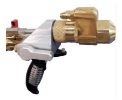
WST water cool jacket is offered as replacement of air cooled jacket to offer colloing of MACHJET-I HVOF gun using cold water from industrial chiller. The jacket has one inlet & one outlet connection for water and has envelope of water around the extended air cap to cool down the jacket parts during HVOF coating operation. Using water jacket offers dense coating and allows coating for long duration. Water jacket is connected to the water jam box module with water hoses.
